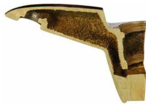
Cross section of brass tap.
