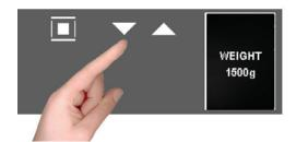
The weight screen appears. Use the  $\blacktriangledown$   $\blacktriangle$  buttons to select the preset values and confirm the choice with the  $\boxed{\blacksquare}$  button.
