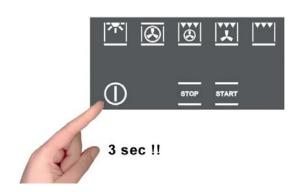
The key function is activated/deactivated by pressing the  $\bigcap$  button for at least 3 seconds.
