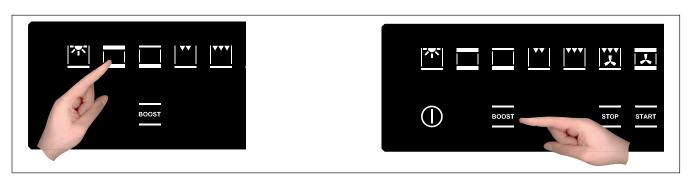
It is possible to disconnect the turbo heat function "BOOST" or change cooking function at any time.
