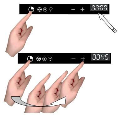
Touch the timer symbol once and the relative symbol will light up. Plus, the clock display will replace the current time:
