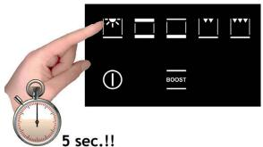
To disable the demonstration mode, touch the light symbol for five seconds: The control will go to normal operation and ready for turning on. Now you can set the time but it is not necessary for turning on the oven.
