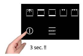
The key function is activated/deactivated by pressing the  $\bigcirc$  button for at least 3 seconds. You can activate and deactivate the operating mode of the oven at any time.
