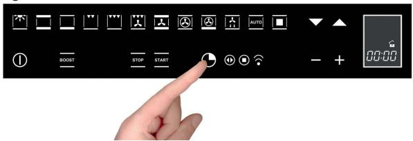
The oven will signal that it is connected to the power mains with a double beep. To set the system time, press the "TIMER FUNCTIONS" button ( ) for at least 3 seconds
