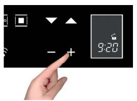
Set the clock with the + and - buttons: during setting the separator dots flash, the time has been set when the dots remain steady on.
