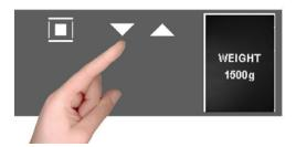
The weight screen appears. Use the  $\blacktriangledown$   $\blacktriangle$  buttons to select the preset values and confirm the choice with the  $\blacksquare$  button.
