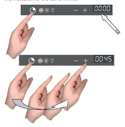
The dividing dots flash to indicate that it is possible to programme the cooking time
