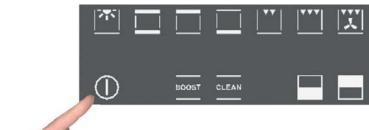
The oven is switched on using the ON/OFF symbol ① shown in the figure. The control activates all the symbols, illuminating the background.
