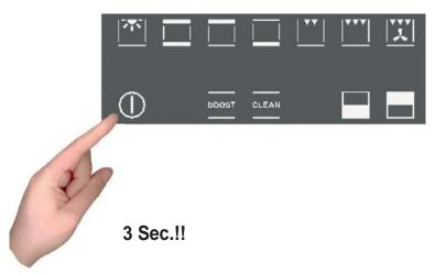
The key function is activated or deactivated by pressing the key ① for at least 3 seconds. It can be activated and deactivated at any time.
