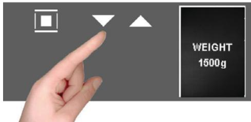
The weight screen appears. Use the ▼ ▲ buttons to select the preset values and confirm the choice with the □ button.
