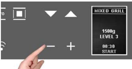
When finished with the settings, the display summarizes the recipe set. The colon in the cooking time (00:30) will be flashing to indicate that it can be changed.
