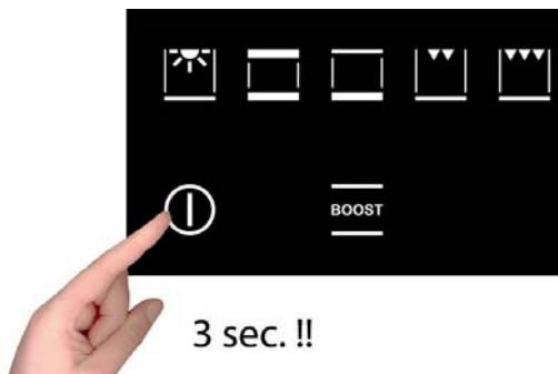
The key function is activated/deactivated by pressing the **I** button for at least 3 seconds. You can activate and deactivate the operating mode of the oven at any time.
