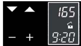
The padlock OPEN symbol means that the key function is not active.
