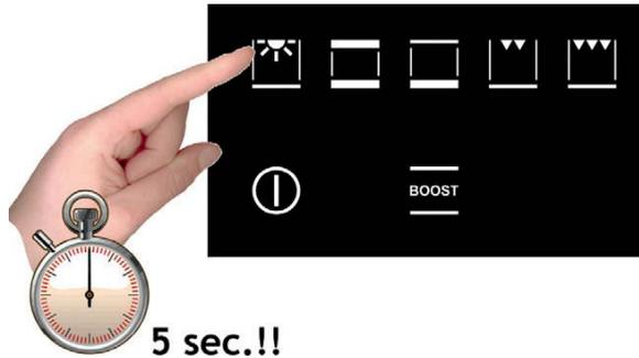
To disable the demonstration mode, touch the light symbol for five seconds:
