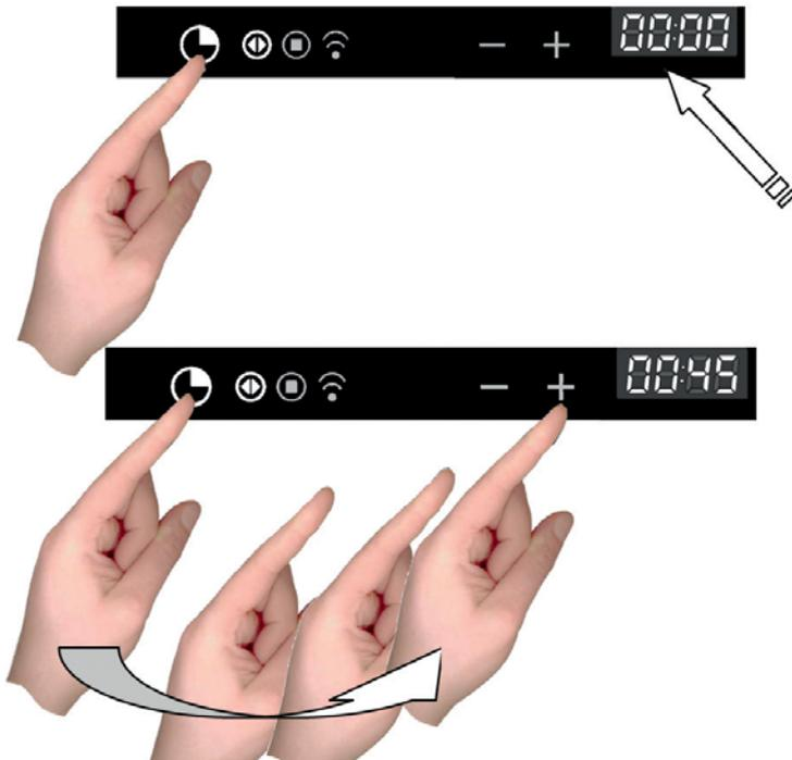
Touch the timer symbol once and the relative symbol will light up. Plus, the clock display will replace the current time:
