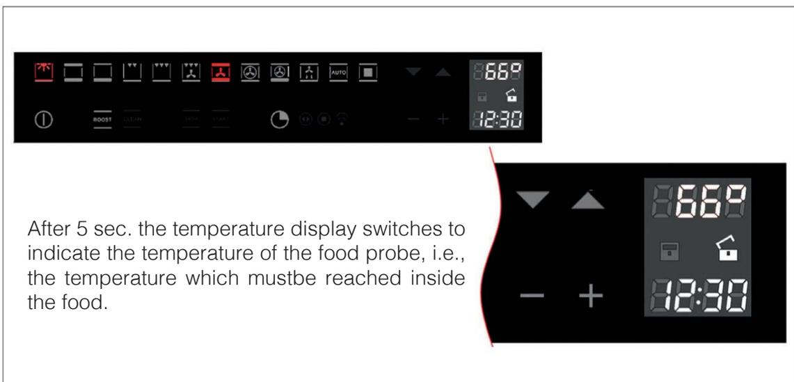
After 5 sec. the temperature display switches to indicate the temperature of the food probe, i.e., the temperature which must be reached inside the food.
