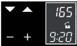
The padlock OPEN symbol means that the key function is not active.
