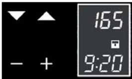
The padlock CLOSED symbol means that the key function is active.
