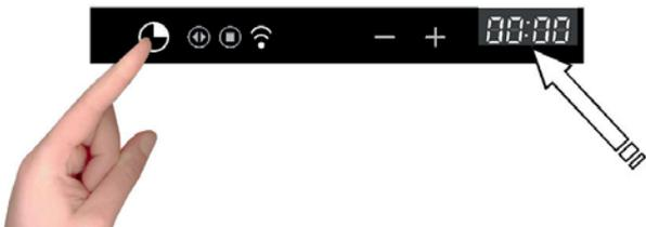
The separator dots flash to indicate you can set the time.
