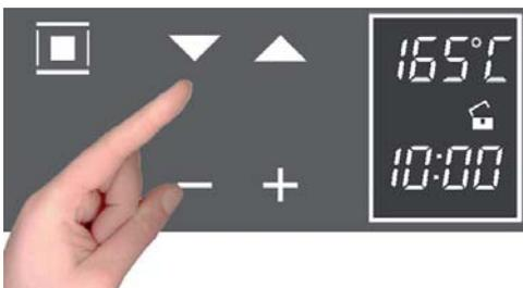
During heating, the centigrade symbol (°C) flashes to indicate that it is heating up to reach the selected temperature. When the temperature is reached, it beeps.
