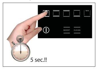
To disable the demo mode, touch the light symbol for five seconds: the controls will enter into standard operational mode and the oven is ready to be switched on.
