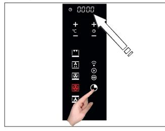
The dividing dots flash to indicate that it is possible to set the value.
