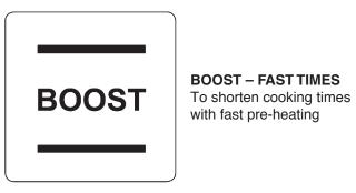
This special function can be activated after selecting a cooking function and is used to reduce the time required to reach the set cooking temperature.
