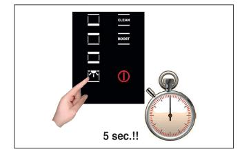
To disable the demo mode, touch the light symbol for five seconds: the controls will enter into standard operational mode and the oven is ready to be switched on.
