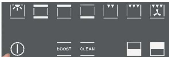
The oven is switched on using the ON/OFF symbol (I) shown in the figure. The control activates all the symbols, illuminating the background.
